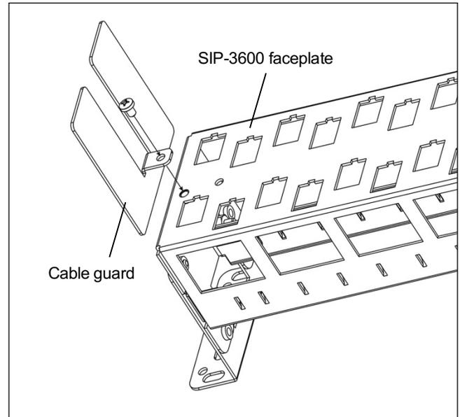
Figure 1. Cable guard attachment to SIP-3600.
